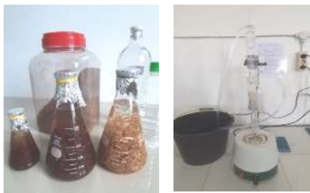
Figure 2. The set up of maceration and soxhletation methods
